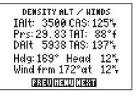
The GPS 95 provides density altitude, true airspeed (TAS) and winds aloft calculators for your convenience. The density altitude and TAS calculations will help you determine critical aircraft performance data.
