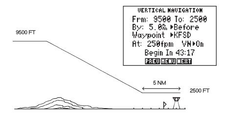
Pilots will find the GPS 95's vertical navigation (VNAV) function useful for calculating vertical speed requirements. In order to use the VNAV feature, aircraft ground speed must be greater than 35 knots.
