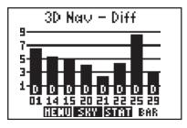
When operating with an RTCM input selected, the Bar Graph Display will denote each satellite for which differential corrections are available with a "D" at the bottom of the bar. (See Section 8.12 for more information on RTCM input selections.) Furthermore, the differential navigation status will also display at the top of the
