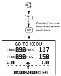
Press the left arrow key to place the cursor on the ground speed field (bottom right).
