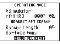
From this page, you may change between various operating modes by highlighting the operating mode field and pressing CLR. You may select simulator mode, normal mode, battery saver mode or AutoLocate mode. (See Section 1.5 for a description of each mode.)
