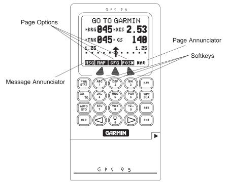
The front panel consists of a 20-key keypad with a 85 x 64-pixel LCD display. Both the display and keypad may be illuminated for nighttime operation.
