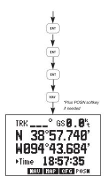
The cursor is over the reference bearing. Since the simulation will begin at LENEX you do not need to define a reference bearing from this point. Press ENT.
