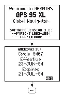
Turn the GPS 95 on. The unit will display the welcome screen and perform several diagnostic checks to ensure that proper operation will occur.
