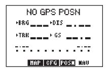
If the GPS 95 has acquired satellites, but is not navigating to a waypoint (i.e., no GOTO destination or route has been activated), the top line of the Navigation Summary Page will indicate that no destination has been defined, as illustrated below.
