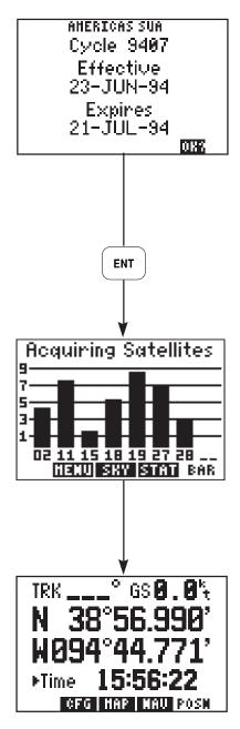
Following completion of the tests, the Database Page will display the effective date, cycle and expiration date of the database. The GPS 95 will still function with an expired database; however, you must exercise extreme caution and always verify that the database information is correct before use. (WARNING: The accuracy of the data is assured only if current. Pilots using an out-of-date database do so entirely at their own risk.)
