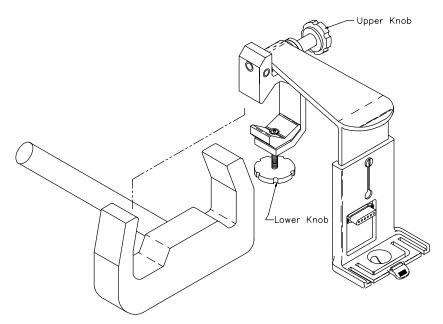
The yoke mount clamp will need to be reconfigured in order to fit the following: Bonanza, Baron and some other Beech models with center column control.
