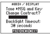
From the Audio/Display Page you can turn the message and/or keypad tones on and off, change the display contrast and change the time-out for the display backlighting.
