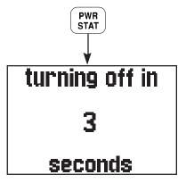
To turn the GPS 95 off, press and hold the PWR/STAT key.
