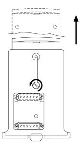
The yoke mount has been designed for easy insertion and removal of your GPS 95 if you wish to use the unit in another airplane or vehicle, to plan at home, or to prevent theft.
