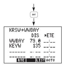
Press ENT to activate the route. The Active Route Page is displayed. This page displays the "active from" and "active to" waypoints on line one, as well as distance and time information to each waypoint on the following lines. The time information is blank since you are not moving yet.
