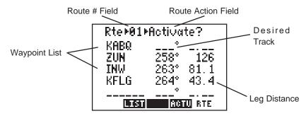
On the route number field, you may choose between routes 0 through 19 with CLR. Next to this is a route action field which allows you to activate the route, clear the route, copy the route to another location, or invert the order of the waypoints in a route and activate it. The arrow keys allow you to scroll through the list of waypoints in a route.
