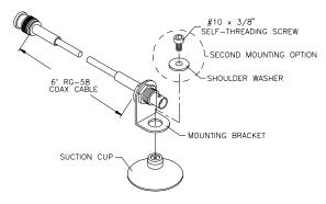
NOTE: The supplied portable antenna mount uses RG-58 coax cable. Modification of this accessory is not recommended, as such modification may adversely affect the shielding capabilities of the cable and cause radio frequency interference. If a substitute cable is desired, standard shielded coaxial cable (RG-58 or RG-59 recommended) should be used.
