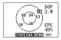
The Satellite Skyview Page shows the azimuth and elevation of each visible satellite in a graphic sky view format. Additionally, DOP and EPE values are shown on the right hand side of the page. The display is always oriented "north up" and is useful in determining whether a satellite signal is being blocked by part of the aircraft, buildings,
