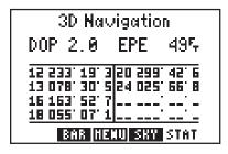
The Satellite Status Page shows the ID, azimuth, elevation, and signal quality of each visible satellite in a table format. The receiver status, again, is displayed at the top of the screen. The second line displays two system quality values dilution of precision (DOP) and estimated position error (EPE). EPE and DOP are advisory information only and are not to
