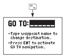
Navigating to a waypoint is easy. Press GOTO and the GPS 95 will display the GOTO Page, as illustrated. Notice that the cursor is to the right of "GOTO". On this field you will enter the identifier of your destination waypoint, KCOU.
