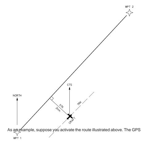
95 chooses the closest leg with a desired track of 45 degrees but your position happens to be two nautical miles off course. The unit will automatically compute the optimal course to steer (which is due north in this example). Press the NAV key until the Nav Summary Page is displayed, then select "CTS" on the first cyclic field. Using the CTS direction (000°), turn so that the track (TRK) and CTS direction match.
