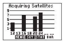
The GPS 95 continually monitors the status of the satellites it tracks and shows that information graphically on a Bar Graph Page. Satellite numbers (1-32) are represented along the bottom of the graph; signal strength (1 to 9, weakest to strongest) is represented along the side. Once a satellite is received, a bar is displayed showing
