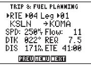
The Trip and Fuel Planning Page allows you to calculate time and fuel requirements between any two waypoints or for any programmed route. On the first cyclic field, you will choose between waypoint (WPT) or route (RTE) planning by highlighting and pressing CLR. If route planning is
