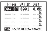
The last field on the Beacon Receiver Setup Page is the "View Beacon Log?" confirmation field. Pressing ENT on this field will display the Beacon Log Page which lists the last five frequencies you have attempted to tune.
