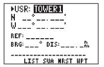
When a waypoint identifier has been entered that does not exist in memory the GPS 95 will assume you wish to create a new waypoint. You may create a new waypoint using one of two methods: direct position entry (latitude/ longitude or grid system) or relative to an existing waypoint.
