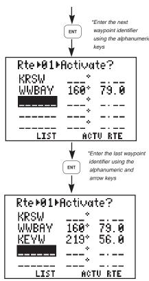
waypoint identifier<br/>using the alphanumeric<br/>keysEnter the identifier for the Whitewater<br/>waypoint (WWBAY) using<br/>the alphanumeric and arrow keys.tte?Press ENT when complete. The cursor<br/>is now on the third waypoint identifier<br/>field.
