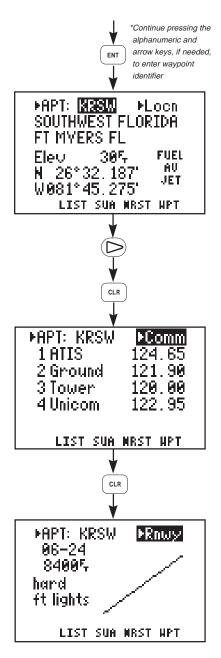
Continue pressing the alphanumeric and, if needed, arrow keys until the waypoint identifier has been entered. Press ENT when complete. Location information will be displayed for the airport (as well as available fuels).
