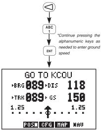
Press the left arrow key to place the cursor on the ground speed field (bottom right).
