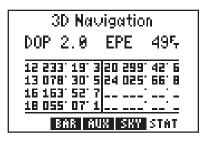
The Satellite Status Page shows the ID, azimuth, elevation, and signal quality of each visible satellite in a table format. The receiver status, again, is displayed at the top of the screen. The second line displays two system quality values dilution of precision (DOP) and estimated position error (EPE). EPE and DOP are advisory information only and are not to
