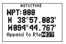
The GPS 95's Autostore<sup>™</sup> feature may also be used to build a route as you are flying. During your flight; as you reach each airport, NAVAID, landmark, or turn to a new heading; you may capture your position and add it to a route. Once you reach your destination you can then invert the route and follow the same course back to where you started. Or, you may want the route for future reference if you wish to make the same flight again.
