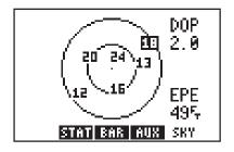
The Satellite Skyview Page shows the azimuth and elevation of each visible satellite in a graphic sky view format. Additionally, DOP and EPE values are shown on the right hand side of the page. The display is always oriented "north up" and is useful in determining whether a satellite signal is being blocked by part of the aircraft, buildings,
