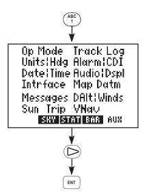
Select the Auxiliary Menu by pressing the AUX softkey (the "1" key in this case).
