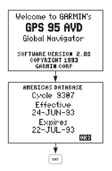
Turn the GPS 95 on. The unit will display the welcome screen and perform several diagnostic checks to ensure that proper operation will occur.
