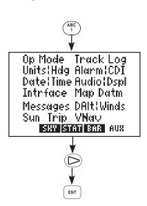
Select the Auxiliary Menu by pressing the AUX softkey (the "1" key in this case).
