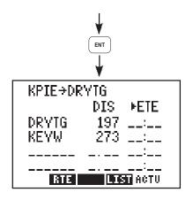
Press ENT to activate the route. The Active Route Page is displayed. This page displays the "active from" and "active to" waypoints on line one, as well as distance and time information to each waypoint on the following lines. The time information is blank since you are not moving yet.
