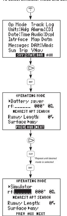
Press the AUX softkey (the "1" key, in this case) to display the Auxiliary Menu.
