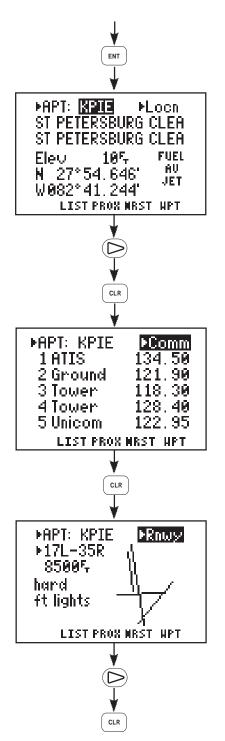
Continue pressing the alphanumeric and, if needed, arrow keys until the waypoint identifier has been entered. Press ENT when complete. Location information will be displayed for the airport (as well as available fuels).
