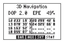
The Satellite Status Page shows the ID, azimuth, elevation, and signal quality of each visible satellite in a table format. The receiver status, again, is displayed at the top of the screen. The second line displays two system quality values - dilution of precision (DOP) and estimated position error (EPE). EPE and DOP are advisory information only and are not to be used as absolute measures of
