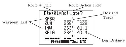
On the route number field, you may choose between routes 0 through 19 with CLR. Next to this is a route action field which allows you to activate the route, clear the route, copy the route to another location, or invert the order of the waypoints in a route and activate it. The arrow keys allow you to scroll through the list of waypoints in a route.
