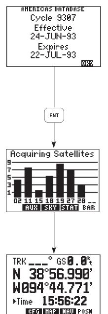
Following completion of the tests, the Database Page will display the effective date, cycle and expiration date of the database. The GPS 95 will still function with an expired database; however, you must exercise extreme caution and always verify that the database information is correct before use. (WARNING: The accuracy of the data is assured only if current. Pilots using an out-of-date database do so entirely at their own risk.)
