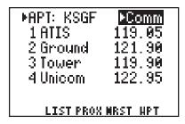
The airport communication information includes identifier (selectable), ATIS, ground, tower and unicom (or multicom) frequencies for the selected airport. Up to five communication frequencies may be displayed at a time. Additional frequencies may be viewed by scrolling.
