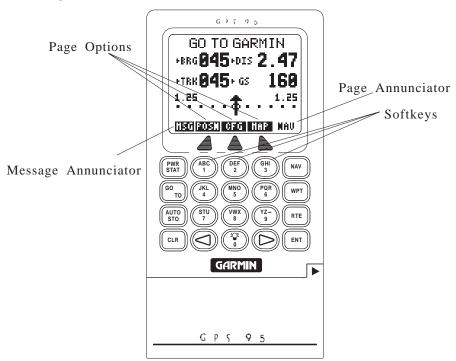
The front panel consists of a 20-key keypad with a 85 x 64-pixel LCD display. Both the display and keypad may be illuminated for nighttime operation.
