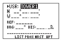
When a waypoint identifier has been entered that does not exist in memory the GPS 95 will assume you wish to create a new waypoint. You may create a new waypoint using one of two methods: direct position entry (latitude/longitude or grid system) or relative to an existing waypoint.
