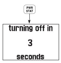
To turn the GPS 95 off, press and hold the PWR/STAT key.
