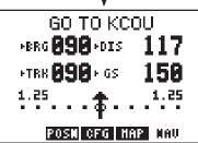
Press the left arrow key to place the cursor on the ground speed field (bottom right).
