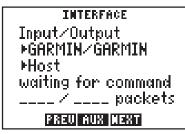
A second cyclic field also appears when the GARMIN input/output is selected. The GARMIN option allows you to exchange data such as waypoints, routes, track logs and satellite almanac data with another GPS 95 or with a PC-compatible computer. You may select between
