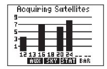
The GPS 95 continually monitors the status of the satellites it tracks and shows that information graphically on a Bar Graph Display. Satellite numbers (1-32) are represented along the bottom of the graph; signal strength (1 to 9, weakest to strongest) is represented along the side. Once a satellite is received, a bar is displayed showing
