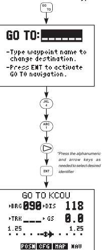
Navigating to a waypoint is easy. Press GOTO and the GPS 95 will display the GOTO Page, as illustrated. Notice that the cursor is to the right of "GOTO". On this field you will enter the identifier of your destination waypoint, KCOU.
