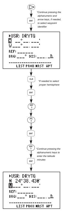
Continue pressing the alphanumeric and, if needed, arrow keys until the waypoint identifier has been entered. Press ENT when complete.
