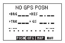
If the GPS 95 has acquired satellites, but is not navigating to a waypoint (i.e., no GOTO destination or route has been activated), the top line of the Navigation Summary Page will indicate that no destination has been defined, as illustrated below.
