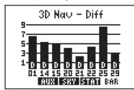
denote each satellite for which differential corrections are available with a "D" at the bottom of the bar. (See Section 8.11 for more information on RTCM input selections.) Furthermore, the differential navigation status will also display at the top of the page. There are two additional receiver status messages available when using
