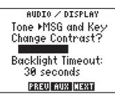
From the Audio/Display Page you can turn the message and/or keypad tones on and off, change the display contrast and change the time-out for the display backlighting.
