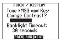
From the Audio and Display Page, you can turn the message and/or keypad tones on and off, change the display contrast, and change the timeout for the display backlighting. Select the desired tone option by highlighting the "Tone>" field and pressing CLR.
