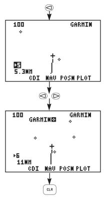
The scale setting is shown in the bottom left corner.
