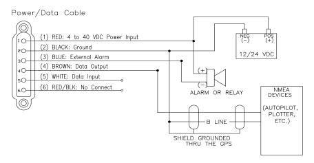
The GPS 75 power/data cable allows you to connect the unit to vehicle power systems, other marine electronics, a remote alarm/beeper, or an external DGPS device that outputs RTCM SC-104, version 2.0 data. The harness will plug into the connector located on the rear panel of the GPS 75.
