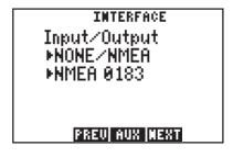
From the Interface Page, you may select the input or output format needed to connect your GPS 75 to other equipment: plotter, autopilot, another GPS 75, a PC, etc. You may select no input/output (NONE/NONE), NMEA output, GARMIN input/output, or RTCM input by highlighting the cyclic field and pressing CLR. When the NMEA
