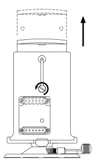
The universal mount is designed to allow the GPS 75 to be installed either with or without the battery pack attached. To adjust the universal mount to accept the GPS 75 with the battery pack attached:
