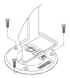
The universal mount is completely assembled and ready for fixed installation above dash. Mount the base to the boat dash using appropriate screws (#8 flat head screws are recommended).
