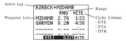
The Active Route Page displays the waypoints of the active route starting with the "active from" and "active to" waypoints on the top line. Press the ACTV softkey to select this page.
