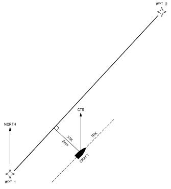
As an example, suppose you activate the route illustrated above. The GPS 75 chooses the closest leg with a desired track of 45 degrees but your position happens to be two nautical miles off course. The unit will automatically compute the optimal course to steer (which is due north in this example). Press the NAV key until the Nav Summary Page is displayed, then select "CTS" on line two. Using the CTS direction (000°), turn so that the track (TRK) and CTS direction match.
