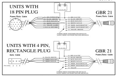
Figure 3 (cont.): Sample Wiring to GARMIN GPS Units
