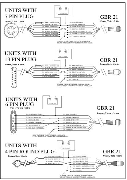
Figure 3: Sample Wiring to GARMIN GPS Units
