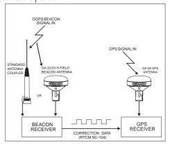
Figure 5: Shipboard DGPS System
