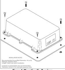
Figure 1: Mounting the Receiver
