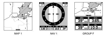
The mapping, navigation, and windows screens above show samples of the AccuMap Sport's three modes. All three are showing navigation data to the same waypoint from the same location. Simply press the MODE key to switch between these screens.
