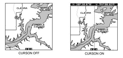
You can move the cursor around the display by pressing the arrow keys in the direction you want it to move. This lets you view different areas of a map, away from your present position. When it's turned on, the zoom-in and zoom-out keys work from the cursor's position - not the present position, so you can zoom in on any detail, anywhere while navigating.
