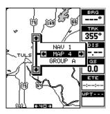
Press the right arrow key to see more screens on each mode. When the desired screen appears, press the EXIT key to clear the menu.
