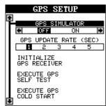
Using the down arrow key, highlight the "Initialize GPS Receiver" menu, then press the right arrow key. The screen shown at right appears.
