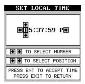
that you want to change. Now press the up or down arrow keys until the desired number shows. Continue until the time shown in the display is correct, then press the ENT key. The unit returns to the navigation, mapping, or windows display with the new time showing.
