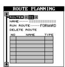
of this screen as shown at right. This is the list of waypoints used in your route. To select the first waypoint in the route, press the right arrow key. A new menu appears as shown below.
