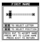
arrow key to move to the next letter. Continue this process until the I.D. is complete. You can press the WPT key to completely erase all of the characters you entered and start over, if you need to. Pressing the EXIT key erases this screen without accepting any input. When the first name is correct, press the ENT key.
