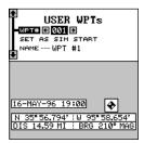
the black box to the "SET AS SIM START" label and press the right arrow key. The AccuMap Sport returns to the Simulator Setup menu.
