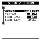
The backlights brightness is also adjustable. To do this, press the up or down arrow keys until the "Light" menu is surrounded by the black box. Now press the left or right arrow key until you have the lights at the desired level. Press the EXIT key when you're finished. The default light level is maximum.
