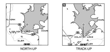
towards the upper right corner of the screen. In the track-up view, the present position moves straight towards the top of the display. A "N" shows to help you see which direction is north when the track-up mode is on. Remember, in the track-up mode, the screen rotates as you change direction. It always keeps your direction of travel (track) heading towards the top of the screen.
