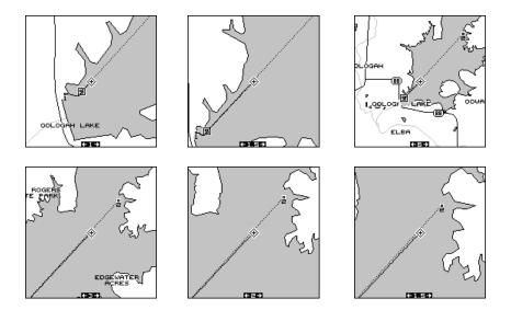
To use the autozoom feature, first set the AccuMap Sport up to navigate to a waypoint. (See the Navigation section for more details.) Next, simply press the MENU key, then use the up or down arrow keys to highlight the "AUTOZOOM OFF/ON" menu. Press the right arrow key to turn it on, the left to turn it off.
