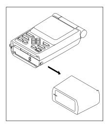
Next, push the battery holder out the bottom of the battery cover as shown below. Install each battery with the negative end (-) against the spring. The positive end (+) of each battery should be firmly against the metal plate. When all six batteries are installed, slide the battery holder into the battery cover.
