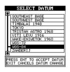
The WGS-84 label is highlighted. To change it, simply press the up or down arrow keys until the desired datum is highlighted, then press the ENT key. This selects the datum and erases the datum menu. The AccuMap 12 is now using the datum you selected.
