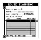
You can place a waypoint using the waypoint list or from locations on the map, or both. For the first waypoint, we'll use the "Insert From WPTS" method. With the black box on this menu, press the right arrow key. A screen similar to the one below appears.
