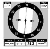
Your speed over ground or Ground Speed is shown at the bottom of this screen. In this example, the ground speed is 21.3 miles per hour. The screen looks like this when you're not navigating to a waypoint. (See page 39 for information on waypoint navigation.) If you navigate to a waypoint, the screen looks like the one below.
