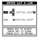
tude number, press the WPT key to erase it and start over. To exit completely out of this screen without saving the position, press the EXIT key.
