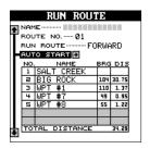
You can start at any waypoint in the route by highlighting the desired waypoint, then pressing right arrow key. A new menu appears as shown at right. The "DIRECT TO" label is highlighted. Press the right arrow key to start the route with this waypoint. To view information (latitude/longitude, distance, bearing, etc.) about this waypoint, highlight the "WPT INFO" label and press the right arrow key. Press the EXIT key to erase the waypoint information menu.
