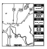
This is Map 3. Your present position is shown as a cross surrounded by a diamond. As you wait for the AccuMap 12 to find your position, you'll see numbers flashing on the display. Anytime you see flashing numbers, it means the AccuMap 12 does not have a position! Do not rely on any data that is flashing! When the numbers stop flashing, the unit has locked on to the satellites and the position is good.
