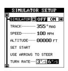
On the example at right, the speed is being changed from 100 m.p.h. to 30 m.p.h.. When the numbers are correct, press the EXIT key.
