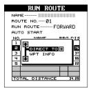
As you travel to the first waypoint, the unit shows navigation data to that waypoint. When you enter the radius around the waypoint set by the arrival alarm, the AccuMap 12 automatically switches to the next waypoint on the list, showing navigation data to that waypoint, and so on until the last waypoint on the route list has been reached. (Note: The arrival alarm does not have to be turned on in order to use the route feature.)
