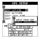
If your latitude is south, press the up or down arrow key to change it. If it is north, press the right arrow key to highlight the first number in the latitude. Now press the up arrow key to increase the number or the down arrow key to decrease it. Once the first number in the latitude is set, press the right arrow key once to move to the next number in the latitude.
