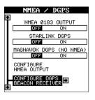
the "Configure DGPS Beacon Receiver" label at the bottom of this screen and press the right arrow key. The screen shown below appears.
