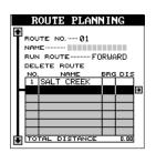
Continue selecting waypoints until the route is complete. As you add waypoints to the list, the bearing and distance from each waypoint to the one previous is shown to the right of the waypoint's name. In this example, the second waypoint in the list is 104 degrees and 30.75 miles from the first waypoint in the list.
