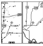
When you press the MENU, ZOOM IN or OUT, or ENT keys, a message appears asking you which display you want to affect. On the screen shown at right, the menu key was pressed. The unit wants to know which map you want to change. Press the left arrow key for the left map, the right arrow key for the right map. The main menu then appears.
