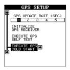
the necessary satellites, but it usually takes less time. Remember, when it does, your local time and possibly date can be wrong. Use the method shown in the initialization section at the front of this manual to change them, if needed. Once this is done, an internal clock will keep the correct time, even when the unit is turned off. The GPS system updates this clock when the unit is locked on to the satellites.
