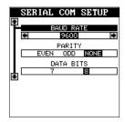
parity, and 8 data bits. Press the EXIT key to erase this menu.
