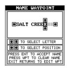
Tip: You can select waypoints by name instead of by number. Simply press the right arrow key while the black box is on the "Name" portion of the waypoint menu, then press the up or down arrow keys until the desired waypoint name appears.
