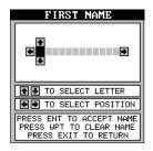
process until the I.D. is complete. You can press the WPT key to completely erase all of the characters you entered and start over, if you need to. Pressing the EXIT key erases this screen without accepting any input. When the first name is correct, press the ENT key.
