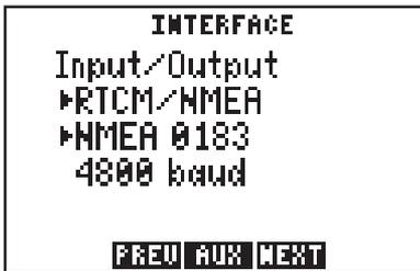
The GPS 95 can use Differential GPS (DGPS) corrections in RTCM SC-104 version 2.0 format. DGPS corrections in this format can be received from an external device (capable of output in 6 to 8 byte format as specified by RTCM SC-104 version 2.0) by connecting the device to the input port on the back of
