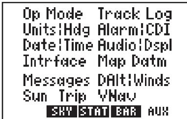
The GPS 95's auxiliary pages allow you to do setup functions to customize your unit and E6-B calculations to plan your flight. The 13 auxiliary pages are accessible from the Auxiliary Menu by highlighting the page you want and pressing ENT. Once an auxiliary page is selected PREV, AUX, and NEXT page options will be displayed. The softkeys
