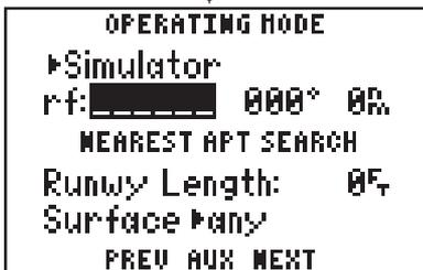
The cursor is now on the reference waypoint identifier. The intersection, LENEX, will be entered here using the alphanumeric keys.
