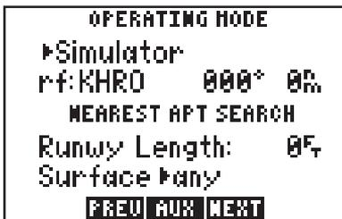
From this page, you may change between various operating modes by highlighting the operating mode field and pressing CLR. You may select simulator mode, normal mode, or battery saver mode. (See Section 1.5 for a description of each mode.)
