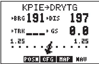
Press the left arrow key to highlight the ground speed field.
