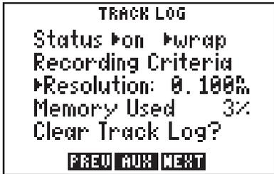
The Track Log Setup Page is used to configure the track log function. A track log is a record of your flight path showing where you have been up to your present position. The cyclic fields on line one allow you to turn the track storage on or off, and determine how the track log will be stored in memory.
