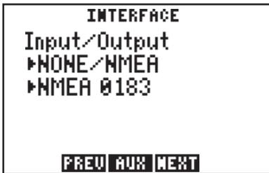
From the Interface Page, you may select the input and/or output format needed to connect your GPS 95 to other equipment: PC, NMEA device, etc. You may select no input/output (NONE/NONE), GARMIN input/output (GARMIN/GARMIN), NMEA output (NONE/NMEA), RTCM input/NMEA output (RTCM/NMEA) or RTCM input (RTCM/NONE).
