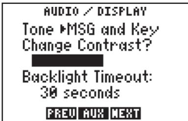
From the Audio/Display Page you can turn the message and/or keypad tones on and off, change the display contrast and change the time-out for the display backlighting.
