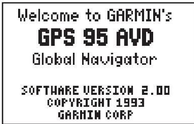
Turn the GPS 95 on. The unit will display the welcome screen and perform several diagnostic checks to ensure that proper operation will occur.
