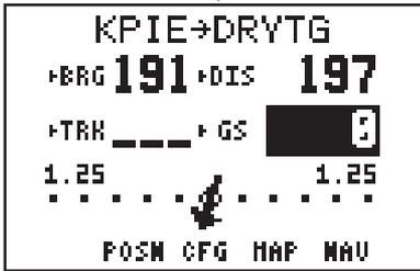
Enter a ground speed of 150 knots. Begin by pressing the "1" key.
