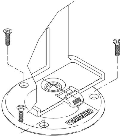
The universal mount is completely assembled and ready for fixed installation above dash. Mount the base to the boat dash using appropriate screws (#8 flat head screws are recommended).
