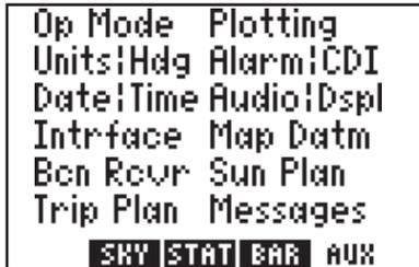
The GPS 75's auxiliary pages allow you to do utility and setup functions to customize your unit. The 11 auxiliary pages are accessible from the auxiliary menu (see Section 3.2) by highlighting the page you want and pressing ENT. The softkeys allow changing to previous (PREV) and next (NEXT) pages. The AUX softkey takes you back to the Auxiliary Menu Page.
