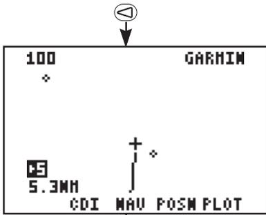
The scale setting is shown in the bottom left corner.
