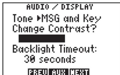
From the Audio and Display Page, you can turn the message and/or keypad tones on and off, change the display contrast, and change the timeout for the display backlighting. Select the desired tone option by highlighting the “Tone>” field and pressing CLR.
