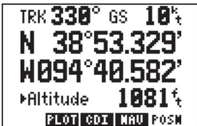
As mentioned earlier, the Position Page is automatically displayed once a position is obtained. This page displays track, ground speed, latitude and longitude relative to the selected map datum (see Section 6.8), as well as a choice of altitude above mean sea level (MSL) or time (cyclic field). (Note: Time information will not be displayed when the GPS 75 is acquiring satellites.)
