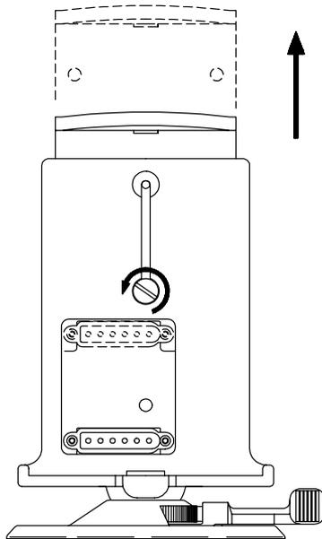
The universal mount is designed to allow the GPS 75 to be installed either with or without the battery pack attached. To adjust the universal mount to accept the GPS 75 with the battery pack attached:
