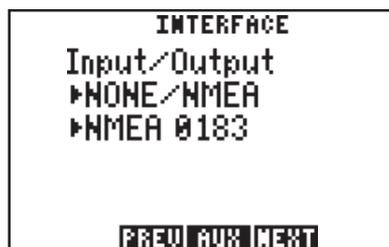
From the Interface Page, you may select the input or output format needed to connect your GPS 75 to other equipment: plotter, autopilot, another GPS 75, a PC, etc. You may select no input/output (NONE/NONE), NMEA output, GARMIN input/output, or RTCM input by highlighting the cyclic field and pressing CLR. When the NMEA
