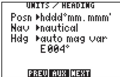
The Units/Heading Page is used to select the units to display for position, distance, speed and heading information. Select the desired position units by highlighting the “POSN” field and pressing CLR. You may choose between degrees only (hddd.dddd°); degrees and minutes
