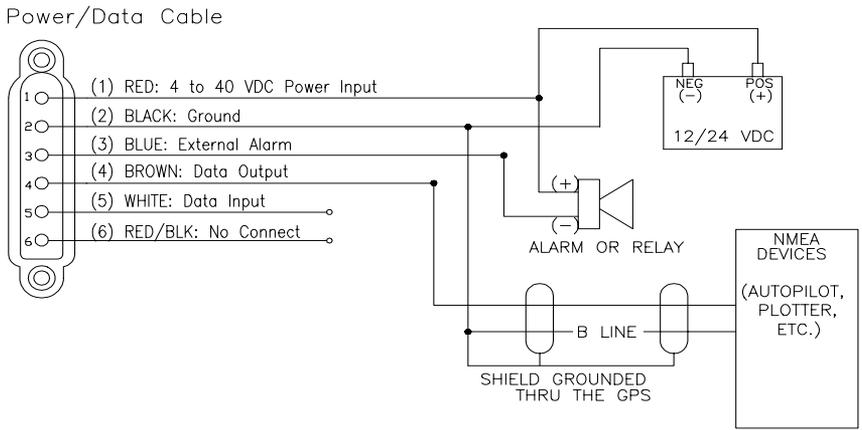
The GPS 75 power/data cable allows you to connect the unit to vehicle power systems, other marine electronics, a remote alarm/beeper, or an external DGPS device that outputs RTCM SC-104, version 2.0 data. The harness will plug into the connector located on the rear panel of the GPS 75.
