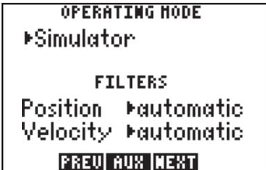
From this page, you may change between various operating modes by highlighting the “OPERATING MODE” field and pressing CLR. You may select simulator mode, normal mode, or battery saver mode. (See Section 2.7 for a description of each mode.)
