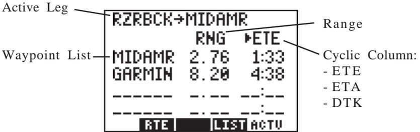
The Active Route Page displays the waypoints of the active route starting with the “active from” and “active to” waypoints on the top line. Press the ACTV softkey to select this page.
