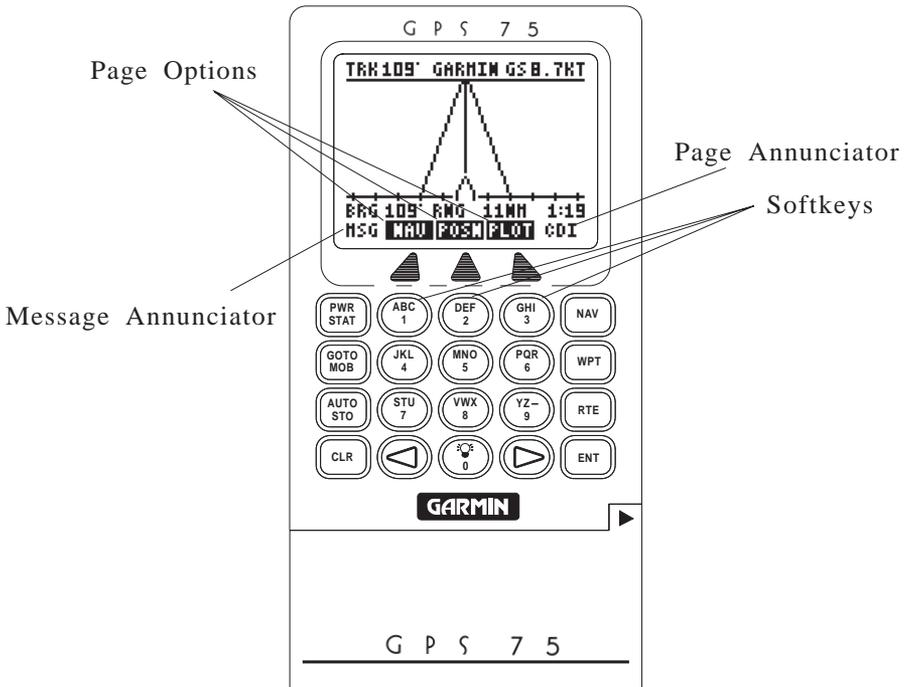
The front panel consists of a 20-key keypad with a 85 x 64-pixel LCD display. Both the display and keypad may be illuminated for nighttime operation.
