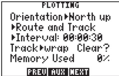
The Plotting Setup Page is used to configure the Plot Page and select the types of information that will be displayed. The first cyclic field defines the orientation of the plot map. The top of the plot map may be North (North Up), the direction of your current ground track (TRK Up), or the direction of the active leg of a
