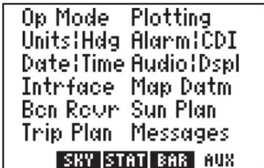
The Auxiliary Menu Page enables the selection of various setup and utility functions by moving the cursor to an item with the arrow keys and pressing ENT. Each setup and utility page is described in detail in Chapter 6.
