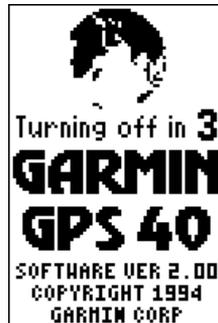
*The power off countdown appears right on screen while you hold the power button. This countdown helps prevent accidental shutoff and loss of data.*
