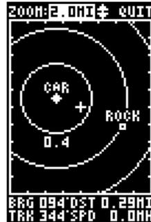
The GPS 40 has on-screen range rings to help you estimate distances relative to your present position. The value of each ring is determined by the current zoom scale.
