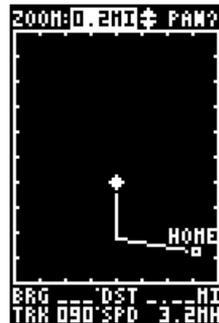
The Moving Map's default setting is track up orientation. It can also be set for north up or desired track up orientation through the map setup page.
