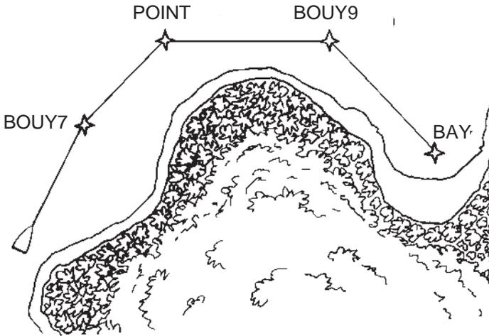
Route 0 is called the active route and is the route used for navigation. The waypoint toward which you are navigating is called the “active to” waypoint. The waypoint immediately behind you is called the “active from” waypoint. The line defined by two consecutive waypoints in a route is called a “leg”. The leg that connects the “active from” and “active to” waypoints is called the “active leg”.
