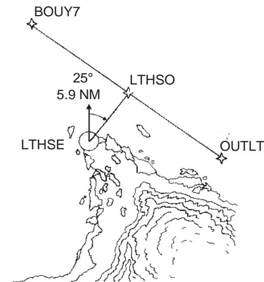
Suppose you are navigating around the coastline of a point with a lighthouse as illustrated above. You need to know when you pass abeam the lighthouse so that you can turn inland but, due to poor visibility, you cannot see the lighthouse. The CPA function will help you find your way!
