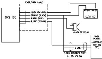
The GPS 100 power/data cable allows you to connect the unit to vehicle power systems, other marine electronics, and a remote alarm/beeper. The harness will plug into the connector located at the left rear corner of the GPS 100.
