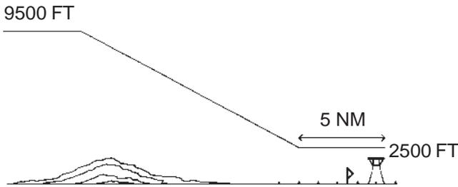
Suppose you are travelling from Denver, Colorado to the Beech factory in Wichita, Kansas. You are flying VFR at 9,500 feet MSL. You wish to be at 2500 feet (500 feet above Beech's traffic pattern altitude) 5 nautical miles from the airport. Additionally, you wish to descend at 1000 feet per minute. Enter the above data on the VNAV Planning page and turn the VNAV function on.
