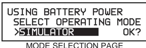
If you are operating the unit with a battery pack or with the battery charger, the above page will be displayed asking you to select the operational mode before proceeding. Recall that you may select Normal, Battery Saver, QuickFix™, or Simulator mode as described in Section 1.4.
