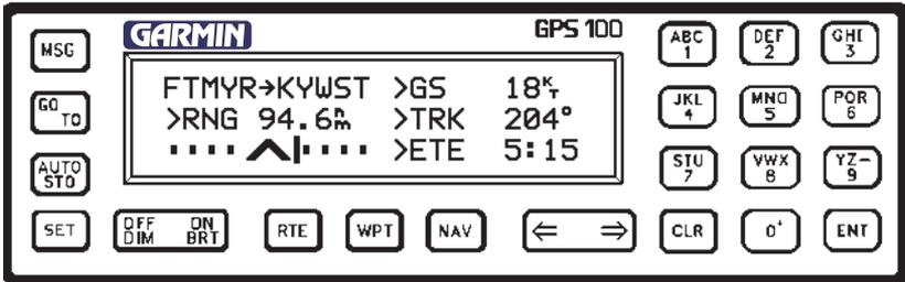
The front panel consists of a 3-line, 22-character LCD display and 21 keys. Both the display and keypad are illuminated for your convenience while operating in the darkness.
