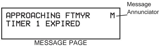
From time to time, the GPS 100 will use a message to tell you of conditions that need your attention. When the GPS 100 has a new message for you, the Message Annunciator will flash. When this occurs, press the MSG key to view new message(s). Continue to press the MSG key until the page you were viewing prior to pressing the MSG key is displayed.
