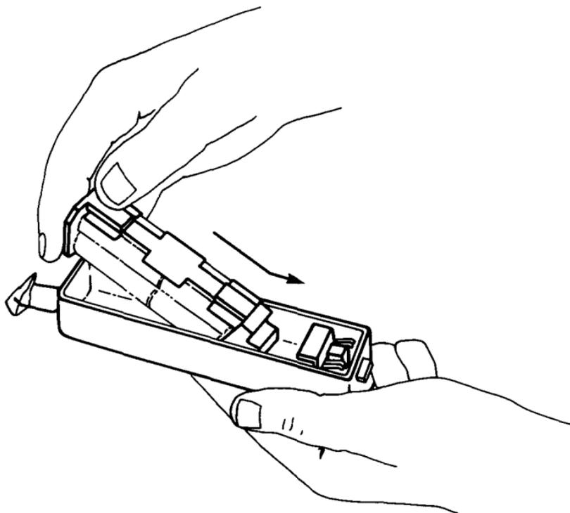
**Removing/Installing the Battery Pack Insert**
