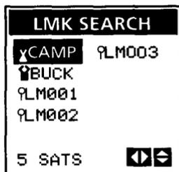
Use the arrow keys to move the highlight bar through the menu. To view landmark coordinates, press **ENTER**.
