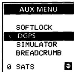
The Trailblazer XL can accept broadcast differential corrections only when it is connected to a compatible differential radio beacon receiver and DGPS is turned on.
