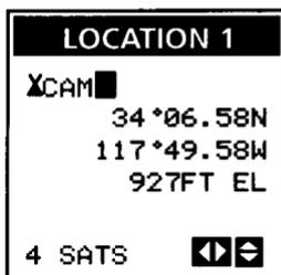
You may enter a message or description that will be saved with the landmark. The message can be displayed when the landmark is viewed from the Landmark Menu and from the navigation screens when the landmark is used in a route. Use the **RIGHT/LEFT ARROW** to highlight "YES" and press **ENTER**. Key in up to 26 characters. Of you do not enter a message now, one can be added later.)
