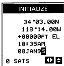
You should not have to re-enter an initial position unless you clear the receiver's memory or move the receiver more than 300 miles from its last location while it is off.
