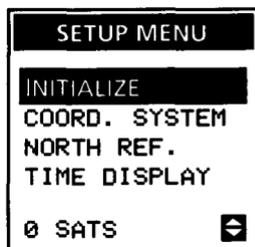
pressing the UP ARROW or the DOWN ARROW will move the highlight bar from one line to the next.
