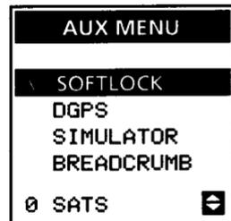
**DGPS.** "DGPS " means "Differential GPS." Differential is a method that reduces the effects of SA to produce highly accurate location fixes. (SA is described in Chapter 5.) The Trailblazer XL can use broadcast differential corrections. This requires the use of a differential radio beacon receiver. Contact your dealer to find out if DGPS is for you and what additional equipment you will require.
