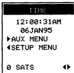
The time displayed by the Trailblazer XL is received from the satellites, then converted to your local dock. Since each satellite carries an atomic clock, the receiver's time is extremely accurate.
