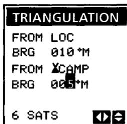
The receiver computes and displays projected coordinates, which can be saved as a landmark by pressing **ENTER**.
