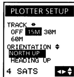
Press the **UP/DOWN ARROWS** to change the orientation of the Plotter from NORTH UP to HEADING UP.
