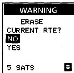
Although you can "overwrite" an existing route, Clearing is a much safer way to remove an unneeded route from the receiver's memory. We recommend that you make a habit of using Route Clear, to help prevent accidentally replacing an important route.
