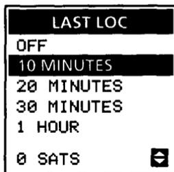
**Sampling.** Sampling turns the receiver on every so often to compute a location fix, save the fix to the buffer, then turn itself back off. You may set the receiver to turn on every 10 minutes, every 20 minutes, every 30 minutes, or every hour. You may also turn Sampling off.
