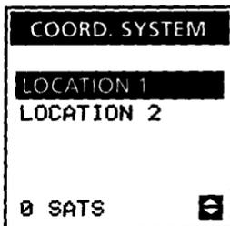
Select the desired coordinate system and press **ENTER**. If you select LAT/LON, you will be asked to select DEG/MIN or DEG/MIN/SEC. Highlight the desired format and press **ENTER**.
