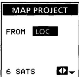
Next, key in the distance north or south from the selected location, then press the **RIGHT ARROW** to move the cursor to the hemisphere. Use the **UP/DOWN ARROW** to display "N" or "S" and press **ENTER**.
