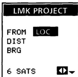
Next, key in the distance from the selected location and press **ENTER**. Key in the bearing and press **ENTER**.
